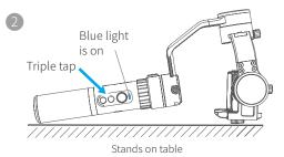
Lay the gimbal on a static flat surface and triple tap the function button. Initialization is successful when the blue light changes from constant on to flashing 3 times periodically.
