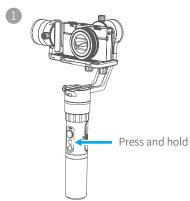
Long press function button and release it until the red light flash, the gimbal enter the standby mode, the blue light will flash 3 times periodically.
