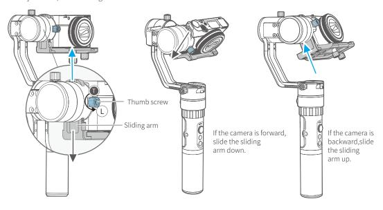
(2) Adjust the center of gravity of the camera's horizontal position in tilting axis.
