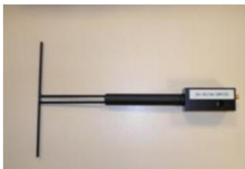
Figure 1 – Satimo COMOSAR Validation Dipole
