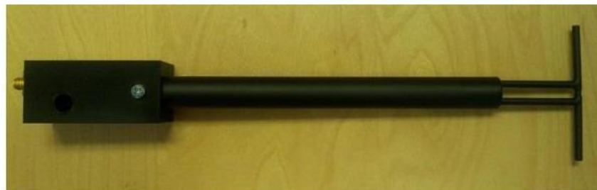
Figure 1 – MVG COMOSAR Validation Dipole
