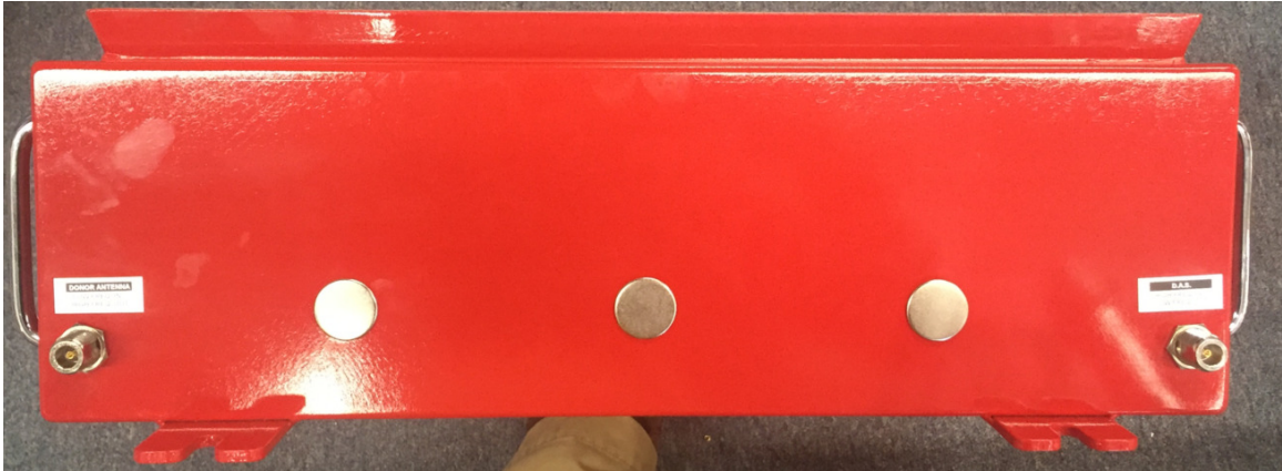
Bottom View With Antenna Ports and Cutouts for Power and Signalling Connections
