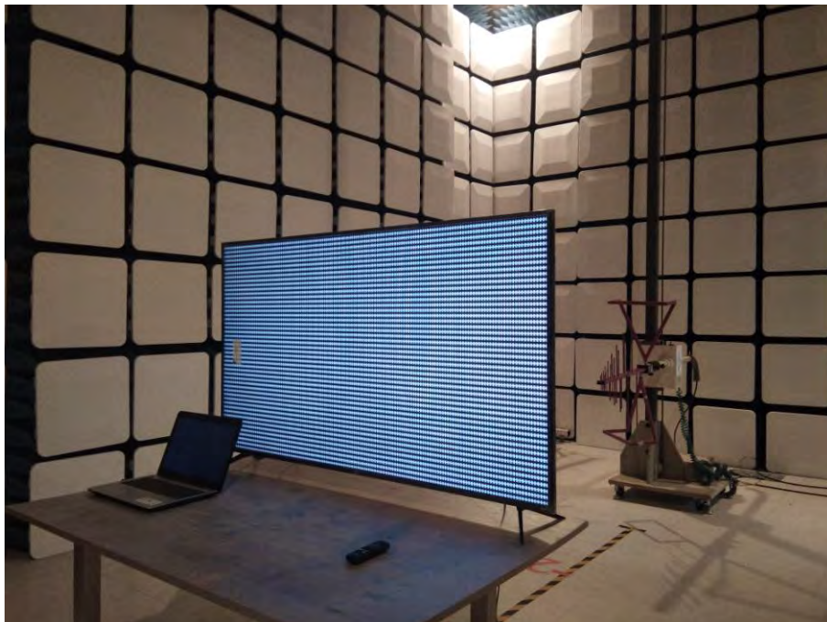
Radiated Measurement Photo 30~1000MHz
