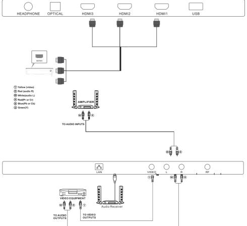
The television's inputs can be connected to the following types of equipment: VCR, multi disc player, DVD, camcorder, video game or stereo system, etc.....
