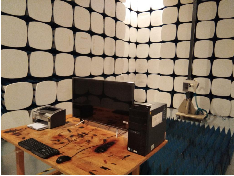
Radiated Measurement Photo 1000~6000MHz
