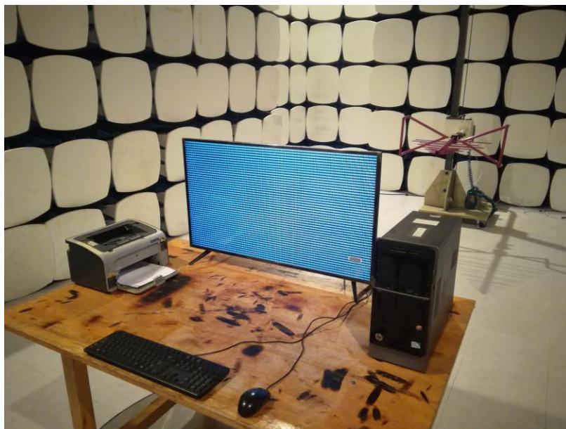
Radiated Measurement Photo 30~1000MHz
