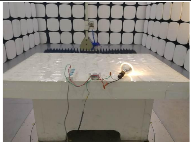
Radiated Emissions Test Setup Above 1GHz
