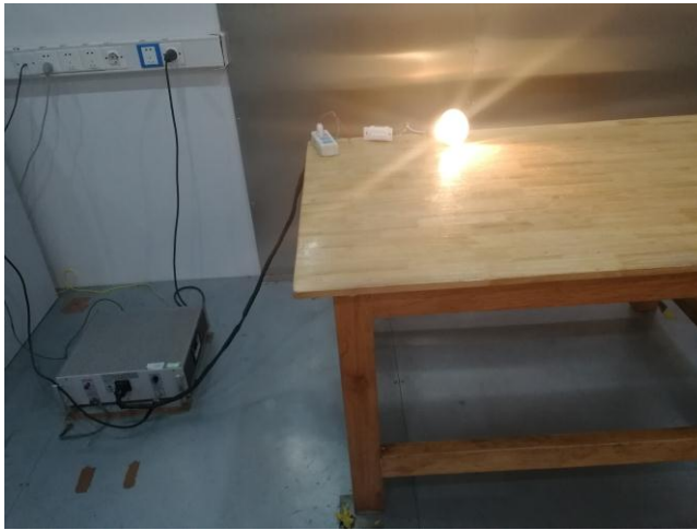
Conducted Emissions Test Setup Front View
