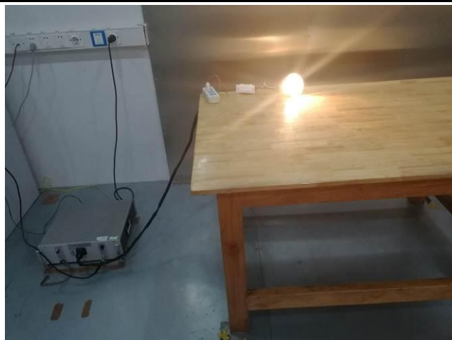
Conducted Emissions Test Setup Front View
