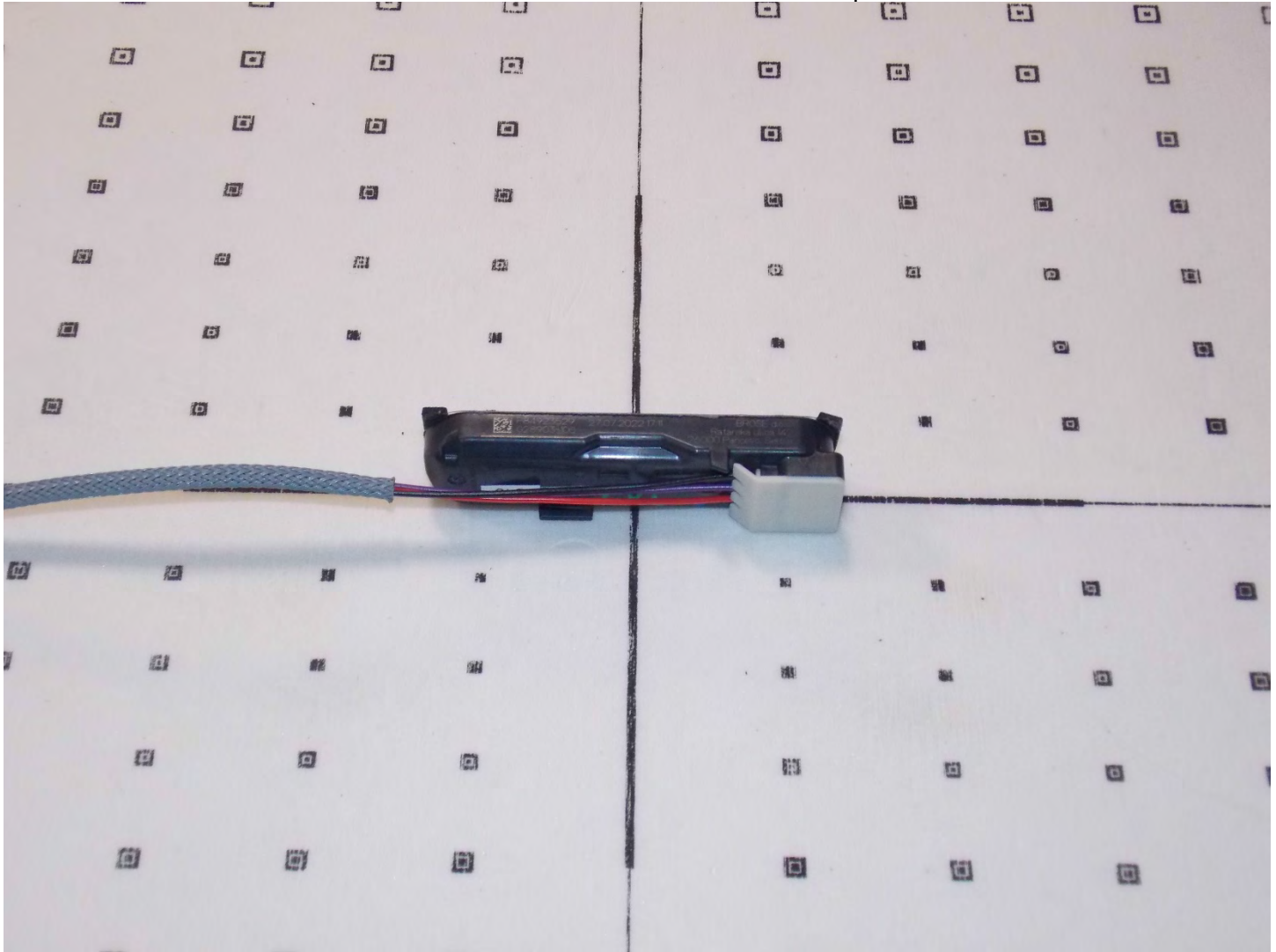
Test Position Right 4.6 mm Gap
