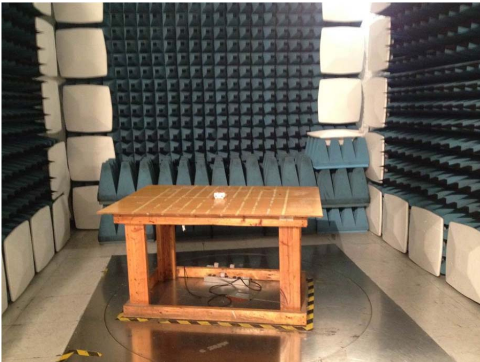
Photograph 2: Radiated Emission Test Configuration, (Below 1GHz) Back
