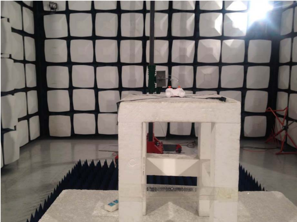
Photograph 3: Radiated Emission Test Configuration, (Above 1GHz) Front
