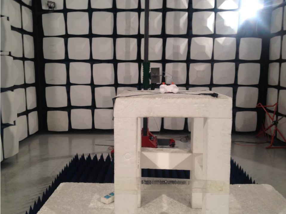
Photograph 3: Radiated Emission Test Configuration, (Above 1GHz) Front
