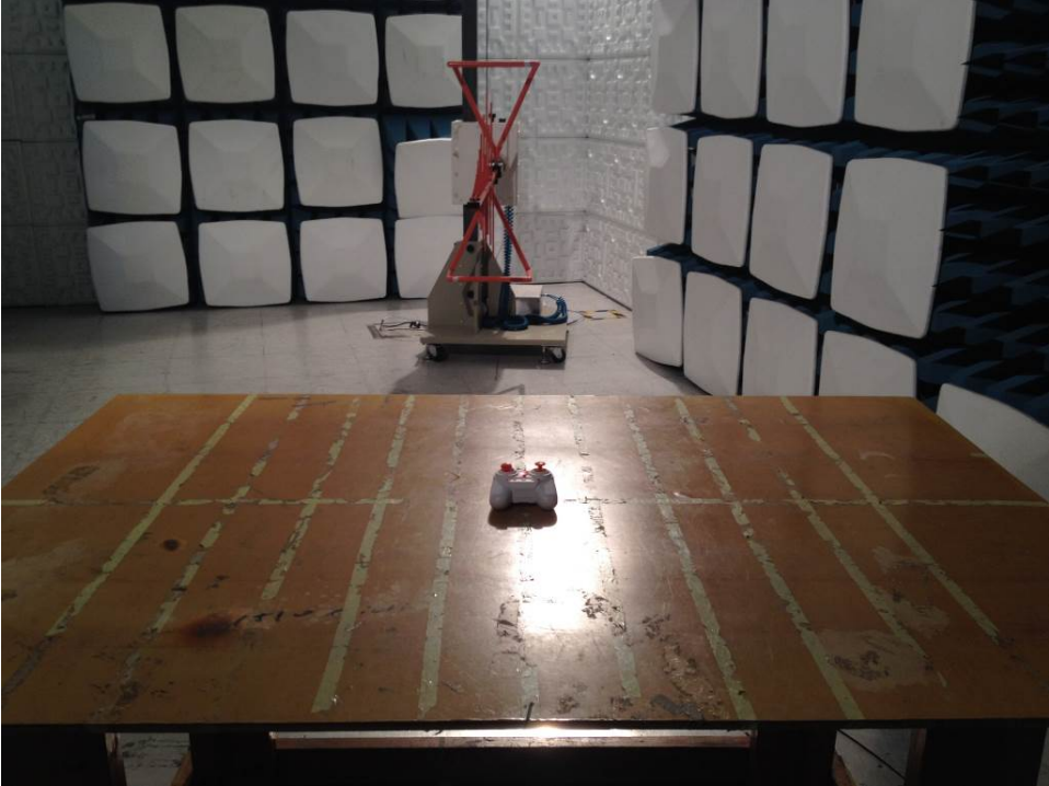
Photograph 1: Radiated Emission Test Configuration, (Below 1GHz) Front
