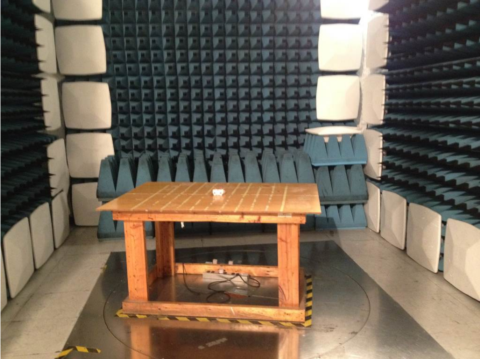
Photograph 2: Radiated Emission Test Configuration, (Below 1GHz) Back
