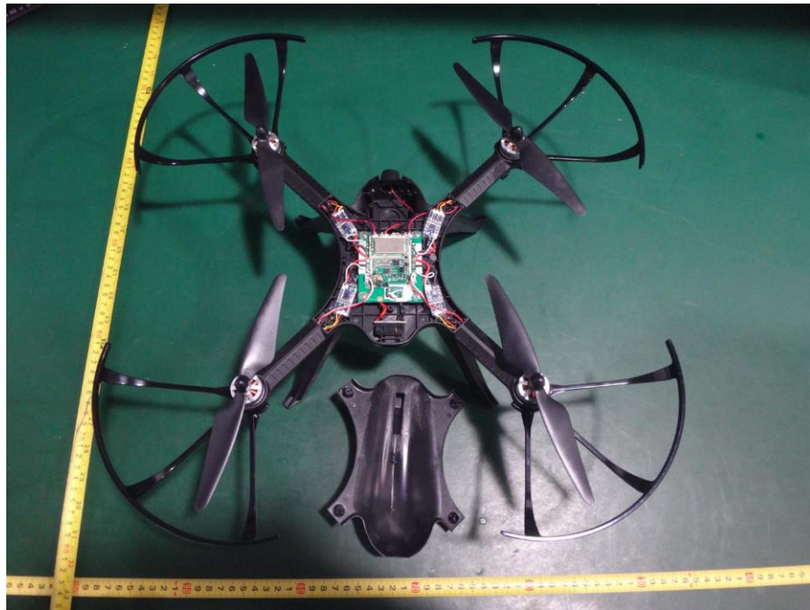
EUT Photo #1 Uncover View
