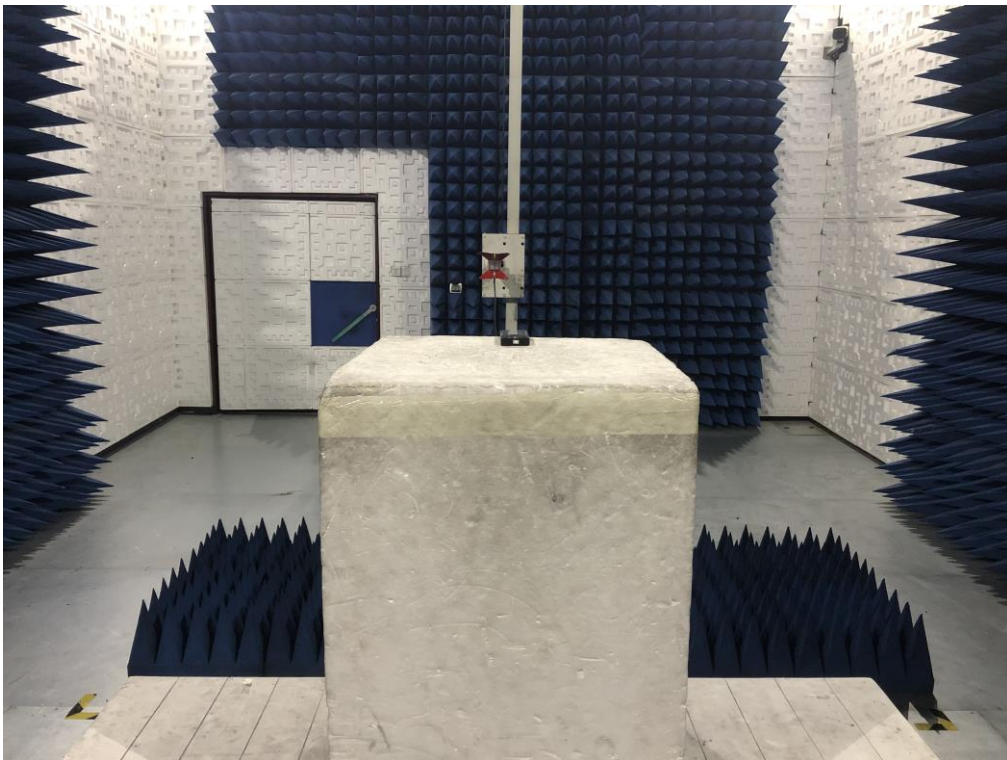
RADIATED EMISSION TEST SETUP ABOVE 1GHZ
