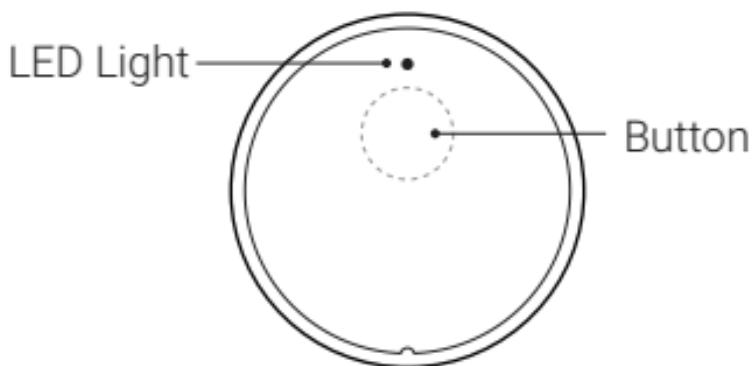
When completing bluetooth connection and the button pressed, LED light is on.
