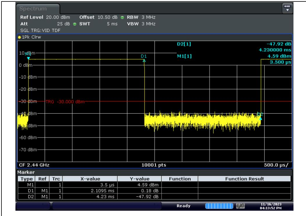
Note 1: Dutycycle factor(dB) :  $10 \times \log(1/(On\text{-time}/Period)) = 3.02 \text{ dB}$
