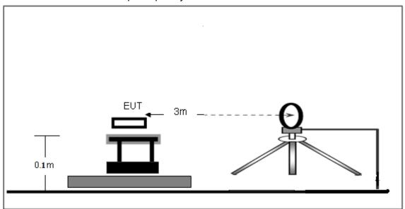
(B) Radiated Emission Test-Up Frequency 30MHz~1GHz
