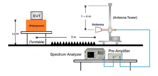
18GHz ~40GHz Test Setup:
