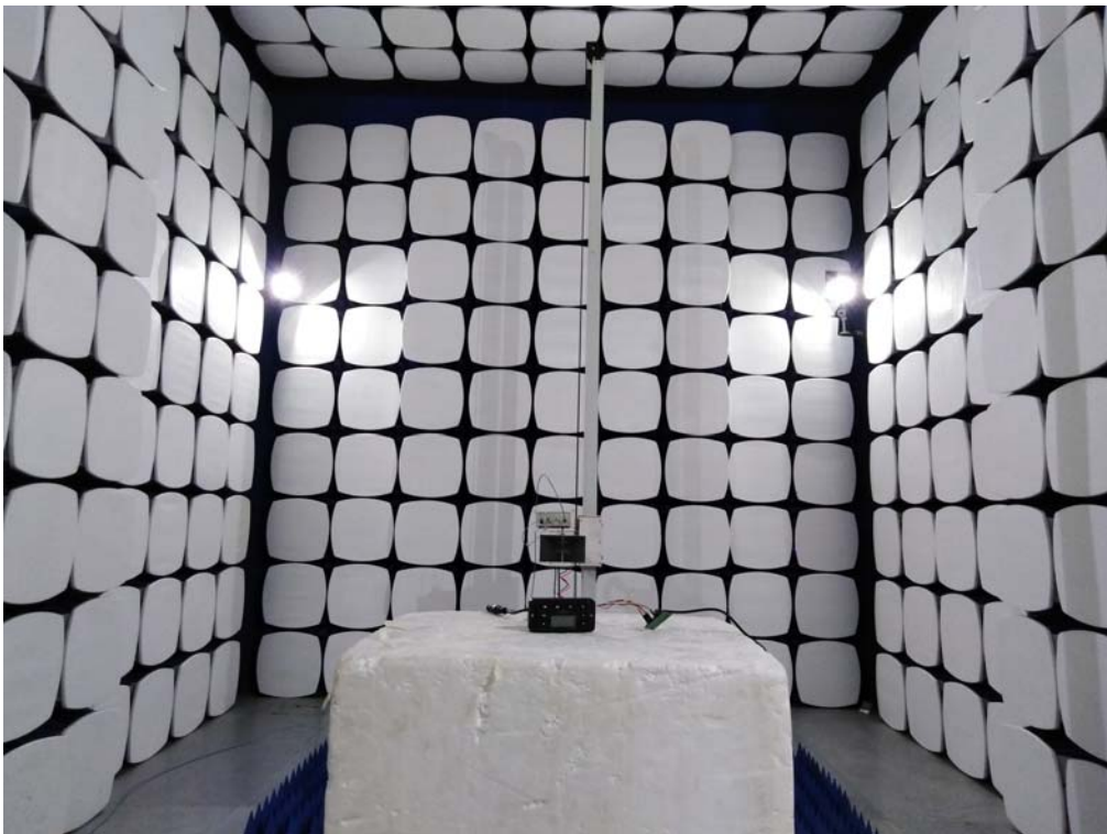
Radiated Setup photo (Above 1G)
