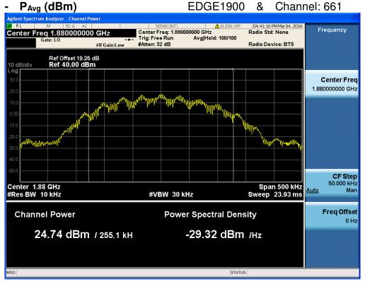
PAR (dB) = P<sub>Pk</sub> (dBm) - P<sub>Avg</sub> (dBm) = 28.10 dBm - 24.74 dBm = 3.36 dB
