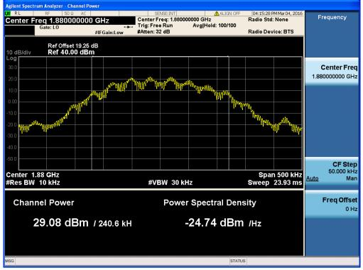
PAPR (dB) = P<sub>Pk</sub> (dBm) - P<sub>Avg</sub> (dBm) = 29.62 dBm - 29.08 dBm = 0.54 dB
