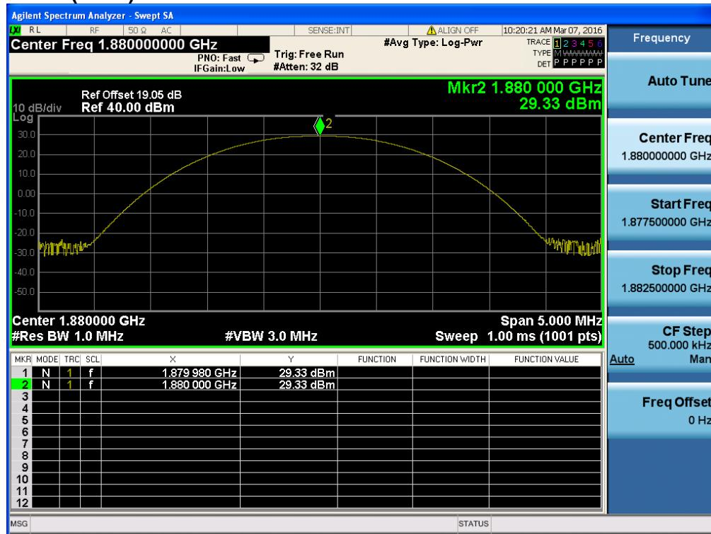
**-P<sub>Avg</sub> (dBm)**      GPRS 1900 & Channel: 661
