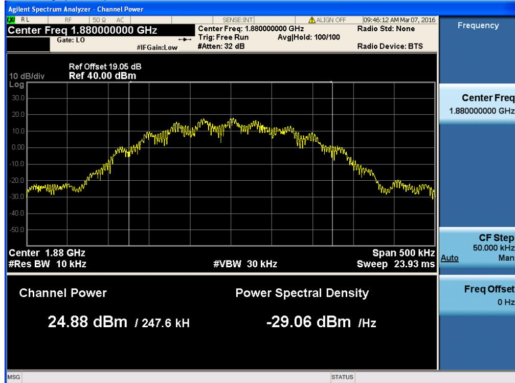
$$\text{PAR (dB)} = \mathbf{P_{Pk} (dBm)} - \mathbf{P_{Avg} (dBm)} = 28.15 \text{ dBm} - 24.88 \text{ dBm} = 3.27 \text{ dB}$$
