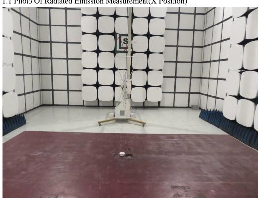
1.1 Photo Of Radiated Emission Measurement(X Position)
