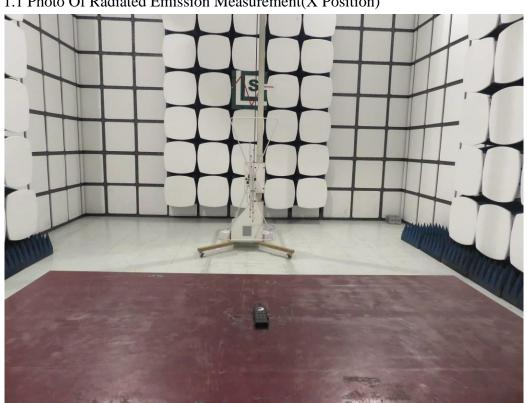
1.1 Photo Of Radiated Emission Measurement(X Position)
