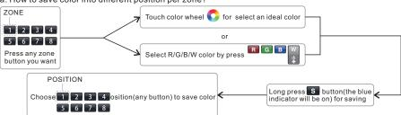
For example, press zone button 1, then touch color wheel for orange color, then press S button (the blue indicator will be on), then choose position button 3. That's to say, we save orange color from zone 1 into position 3. So each zone can save 8 colors. 8 zones can save 64 colors.
