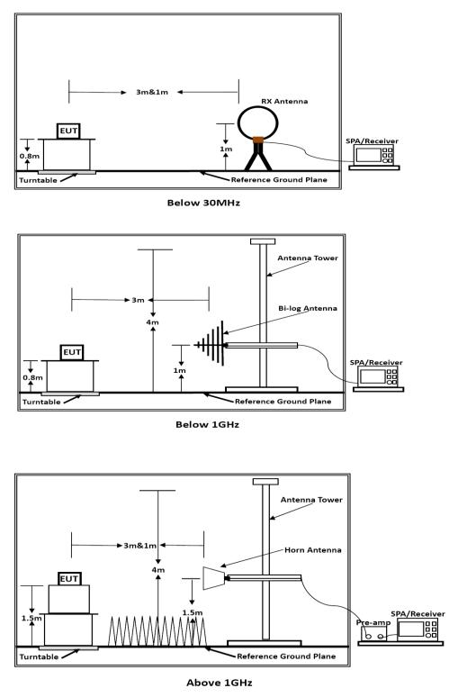
Above 10 GHz shall be extrapolated to the specified distance using an extrapolation factor of 20 dB/decade form 3m to 1.5m.
