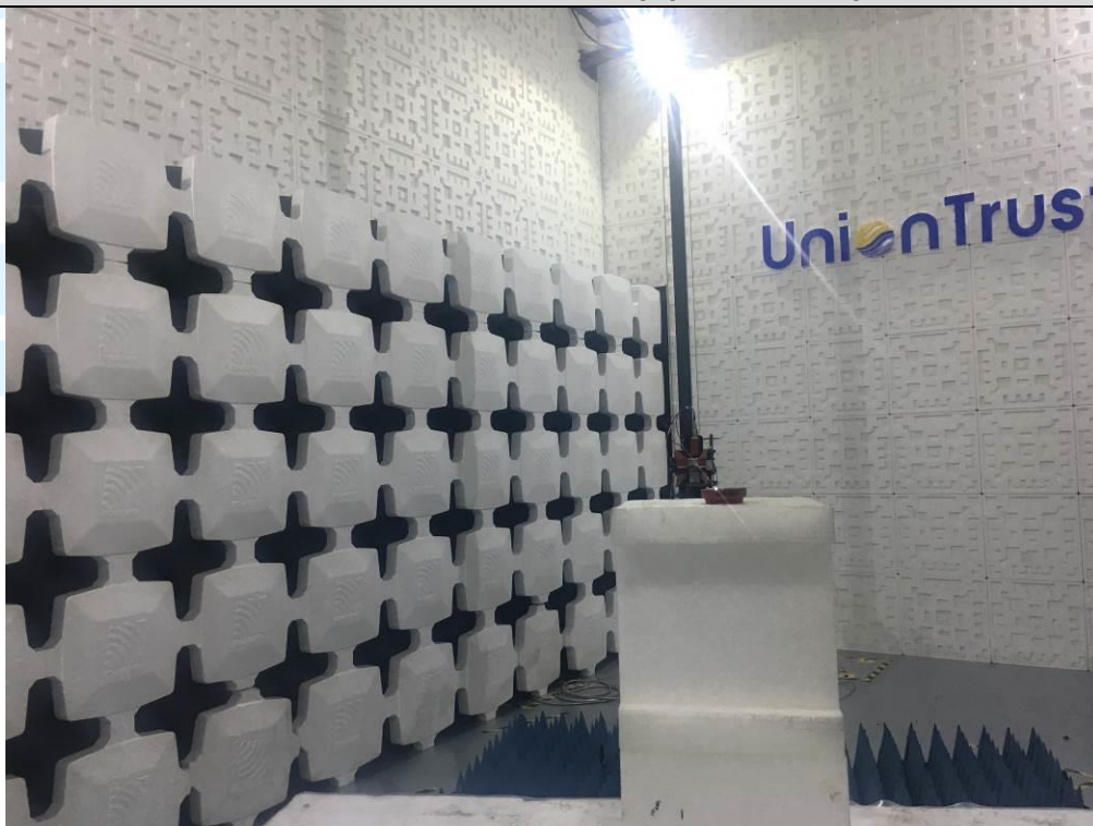
Radiated emission Test Setup (Above 1 GHz)
