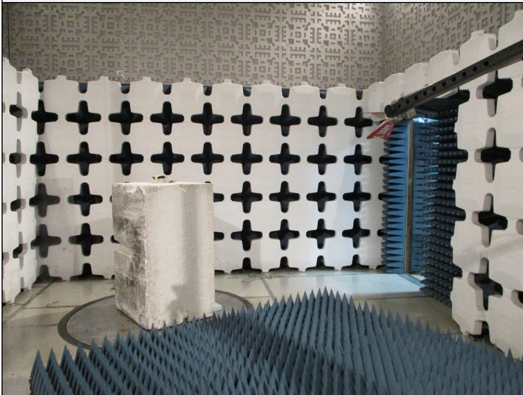
Test Setup for Spurious Radiated Emissions, 1-18GHz – Antenna Polarization Vertical
