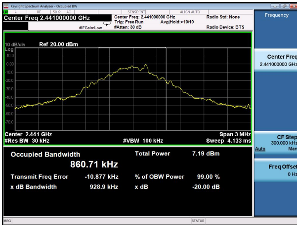
20dB Bandwidth plot on channel 78 (1Mbps)
