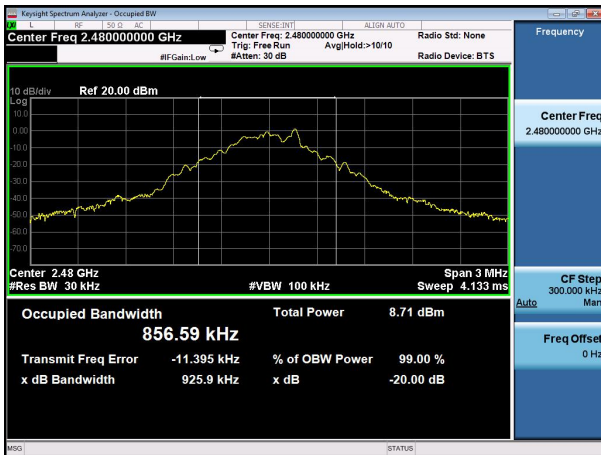
20dB Bandwidth plot on channel 78 (1Mbps)
