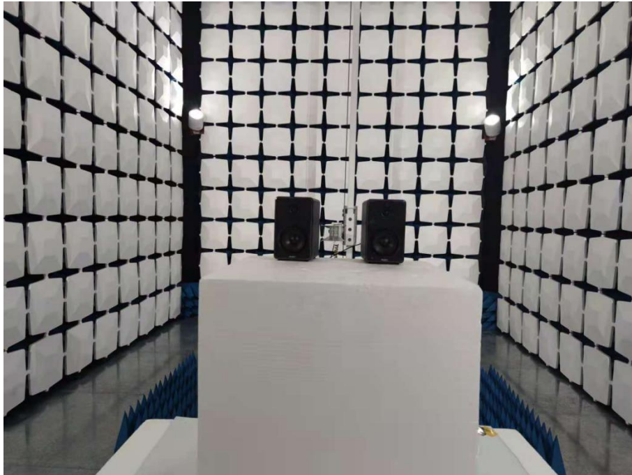
Below 1GHz for radiated emission test setup
