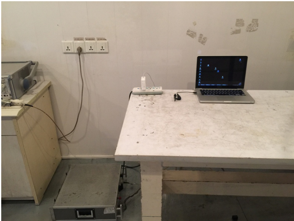
Setup for AC power line Conducted Emission
