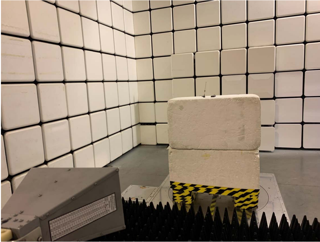
Picture 1: Radiated Spurious Emissions Test setup
