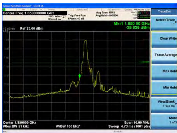
LTE Band 25 3MHz 16QAM 1RB CH-Low
