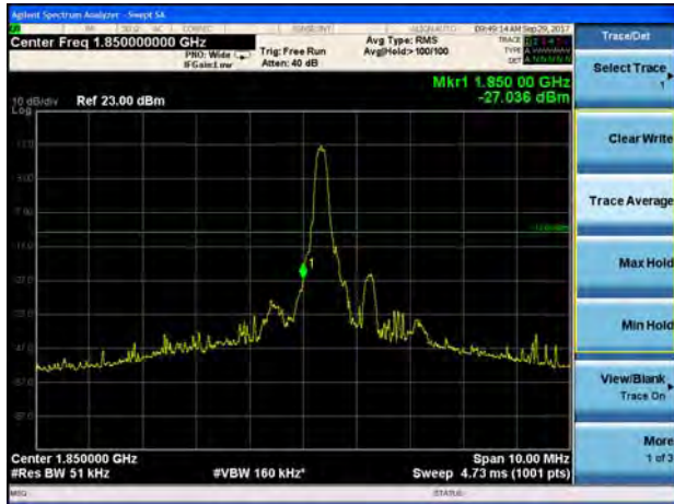
LTE Band 2 5MHz 16QAM 100%RB CH-Low
