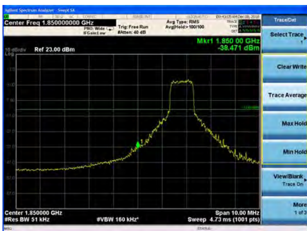
LTE Band 25 20MHz 16QAM 100%RB CH-Low
