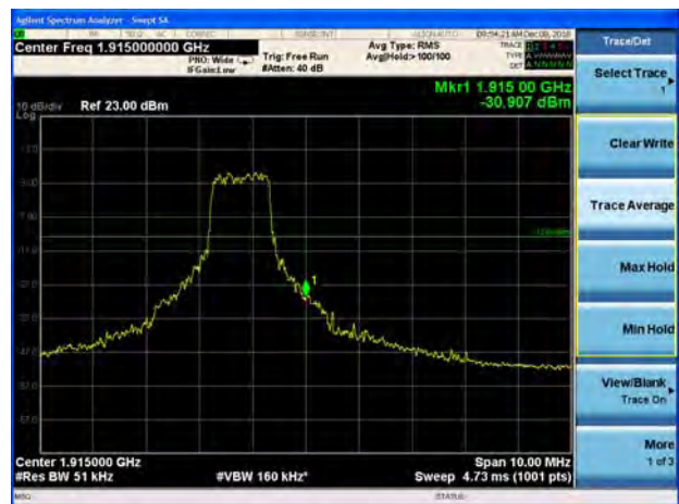
LTE Band 25 15MHz QPSK 1RB CH-High
