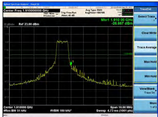
LTE Band 2 10MHz 16QAM 1RB CH-High
