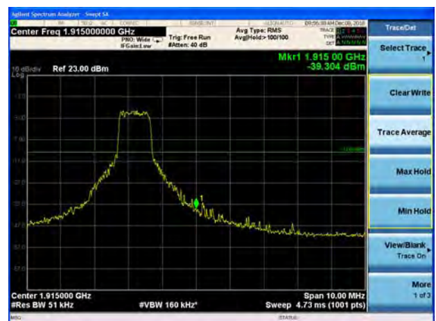
LTE Band 25 20MHz 16QAM 100%RB CH-High
