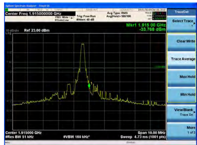
LTE Band 25 3MHz QPSK 1RB CH-High
