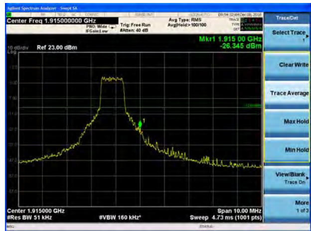
LTE Band 25 15MHz 16QAM 1RB CH-High
