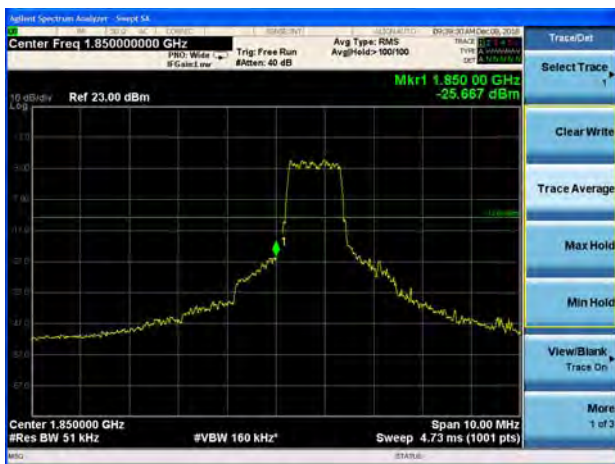
LTE Band 25 5MHz QPSK 100%RB CH-Low
