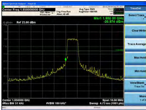
LTE Band 2 3MHz 16QAM 1RB CH-Low
