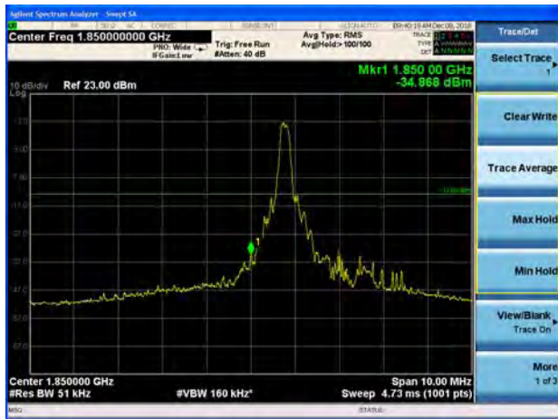
LTE Band 25 10MHz QPSK 100%RB CH-Low
