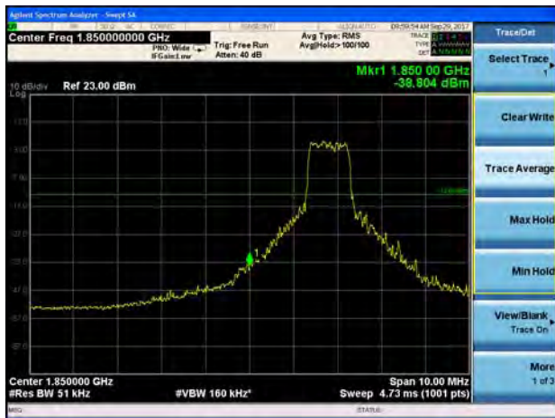
LTE Band 2 20MHz 16QAM 100%RB CH-Low
