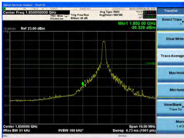
LTE Band 25 20MHz QPSK 100%RB CH-Low
