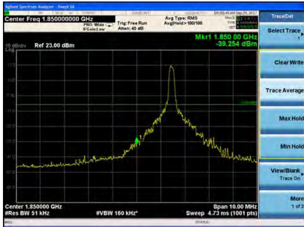
LTE Band 2 20MHz QPSK 100%RB CH-Low
