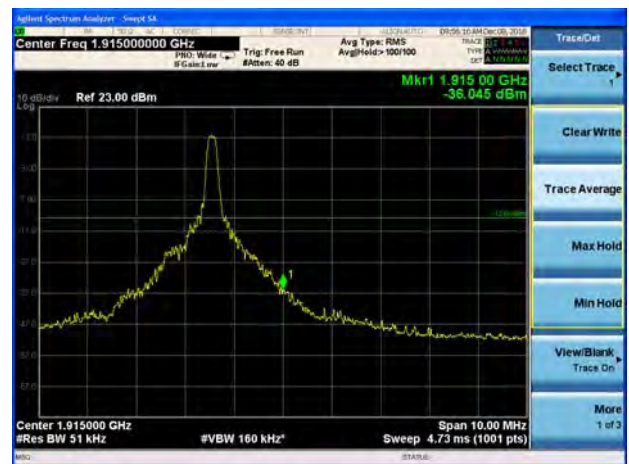
LTE Band 25 20MHz 16QAM 100%RB CH-High
