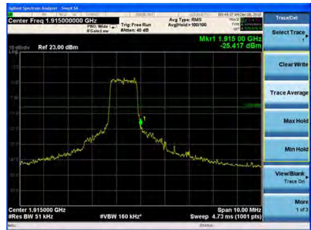
LTE Band 25 3MHz QPSK 1RB CH-High
