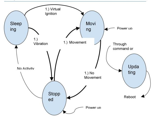
There are 3 main states in the software state machine: Moving, Stopped, Sleeping. There is also an Updating state when the application or settings information on unit are being updated. When in Updating state the device will ignore all normal behavior until unit is updated at which time it is rebooted. The parameters and thresholds applied for state transitions are primarily contained in the Settings File.
