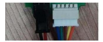
The picture above shows the 2 wire power harness and the 5 wire I/O harness. The wiring details are:
