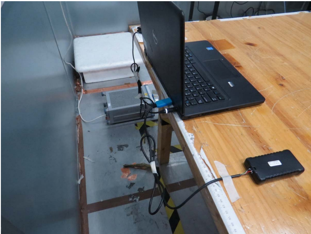
Picture 3 Conducted Emission Test Setup
