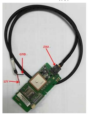
4. The other interfaces of the FJ1000LS device are shown in the following pictures.(The Modem UART 1 on device is for modem debug and update firmware).
