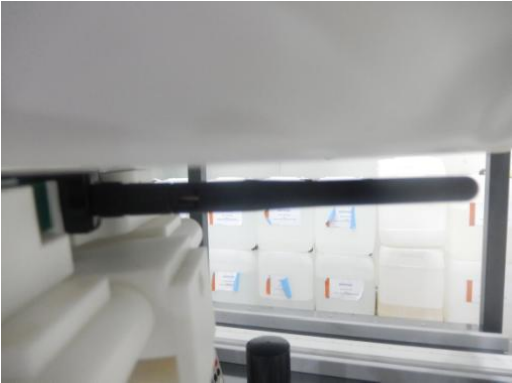
Vertical-Back side(separation distance is 5mm)
