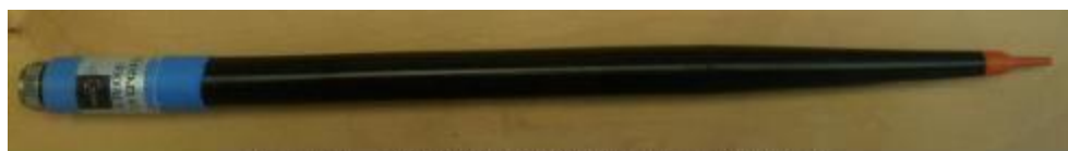
Figure 1 – MVG COMOSAR Dosimetric E field Dipole
