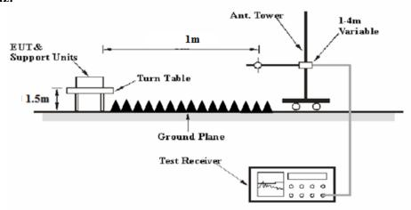
The radiated emission Below 1GHz tests were performed in the 3 meters chamber test site A, above 1GHz tests were performed in the 3 meters chamber test site A, using the setup accordance with the ANSI C63.10-2013. The specification used was the FCC 15.209, and FCC 15.407 limits.
