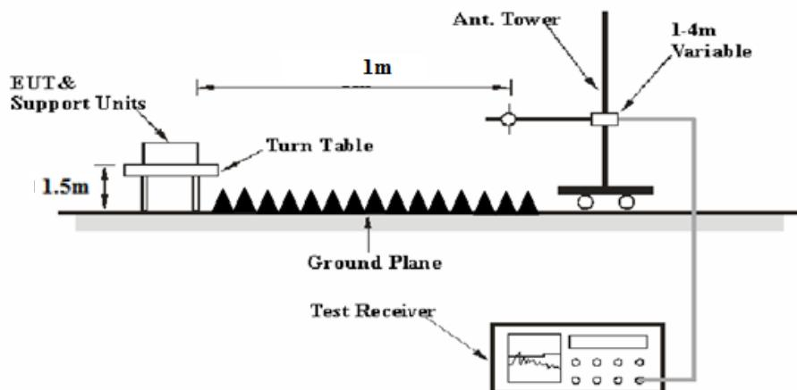
The radiated emission Below 1GHz tests were performed in the 3 meters chamber test site A, above 1GHz tests were performed in the 3 meters chamber test site A, using the setup accordance with the ANSI C63.10-2013. The specification used was the FCC 15.209, and FCC 15.407 limits.
