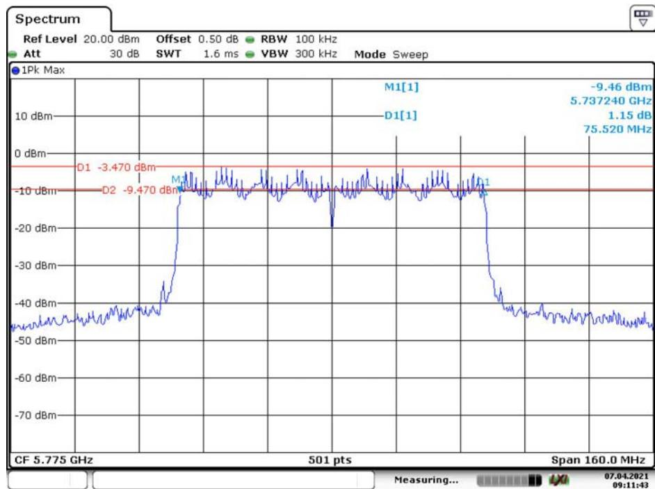
**99% Occupied Bandwidth:****802.11a Low Channel**
