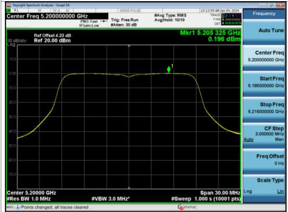
PSD NVNT ac20 5200MHz Ant1
