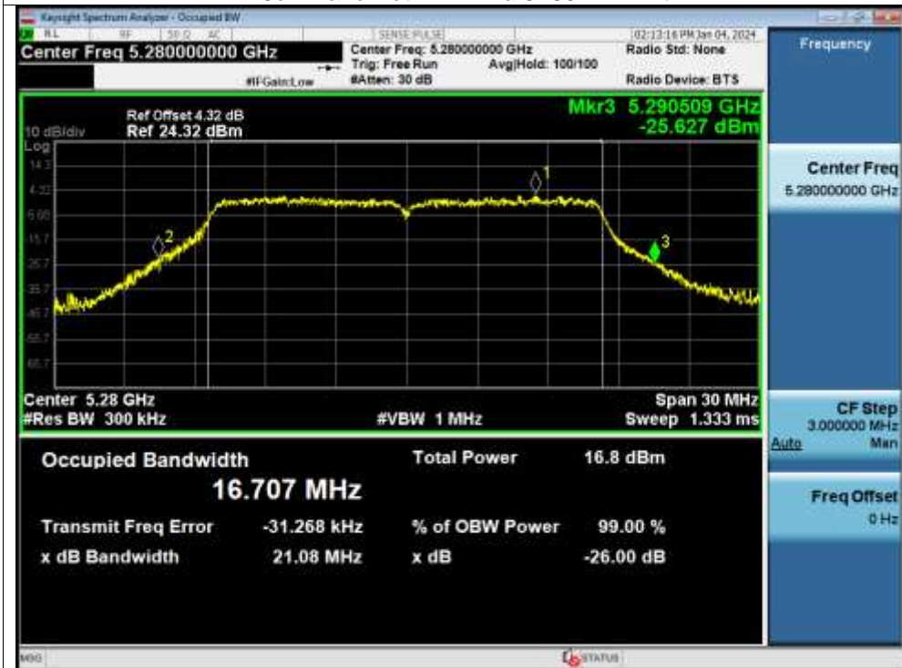
-26dB Bandwidth NVNT a 5280MHz Ant1
