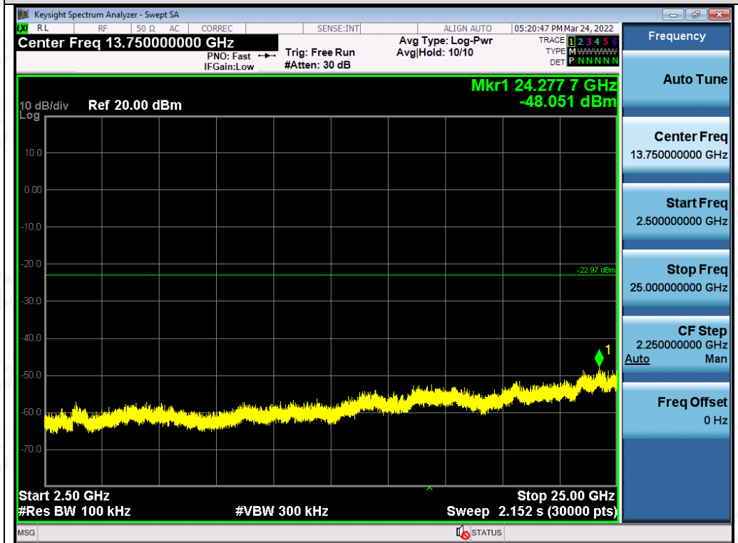
Test_Graph_802.11g_ANT2_2462_6Mbps_Higher Band Emissions
