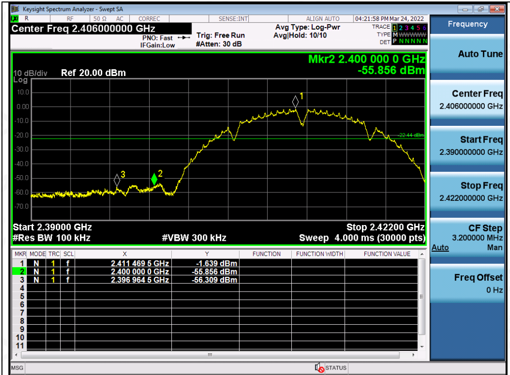
Test_Graph_802.11b_ANT2_2412_1Mbps_Lower Band Edge Emissions
