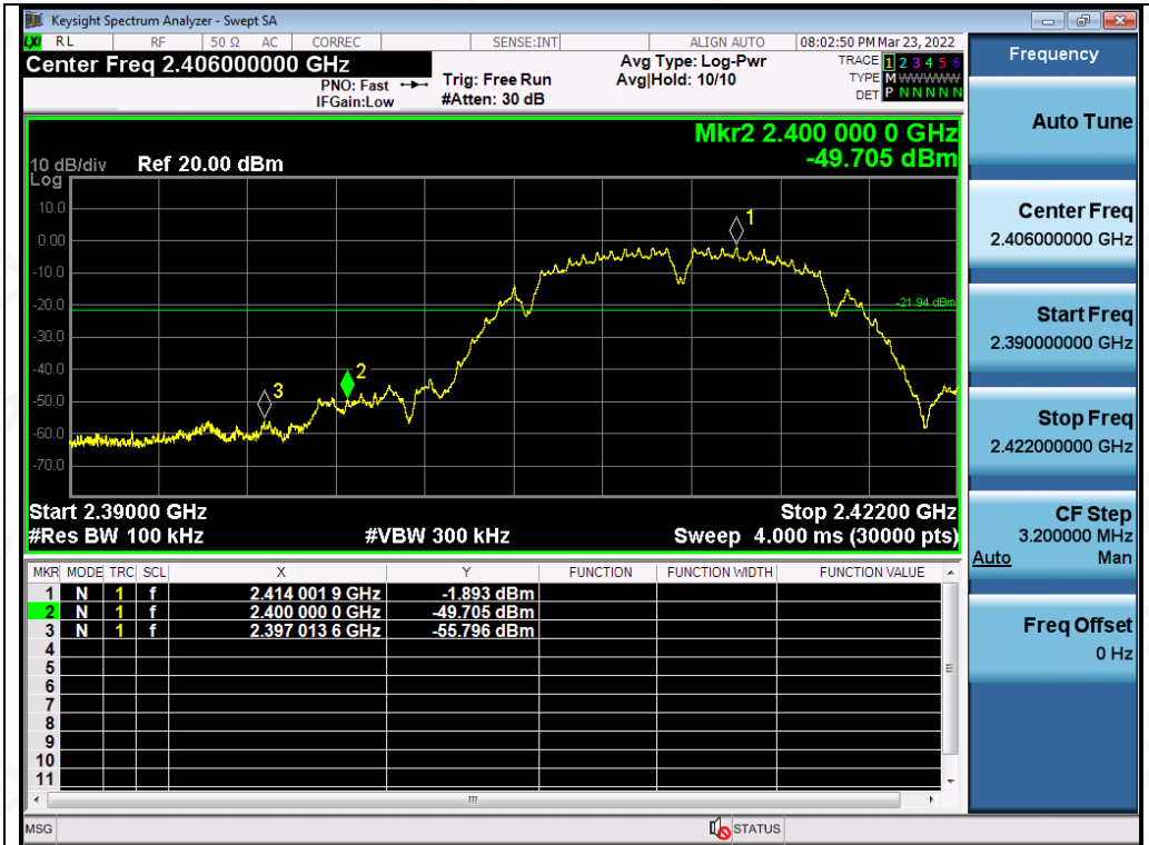
Test_Graph_802.11b_ANT1_2412_1Mbps_Lower Band Edge Emissions
