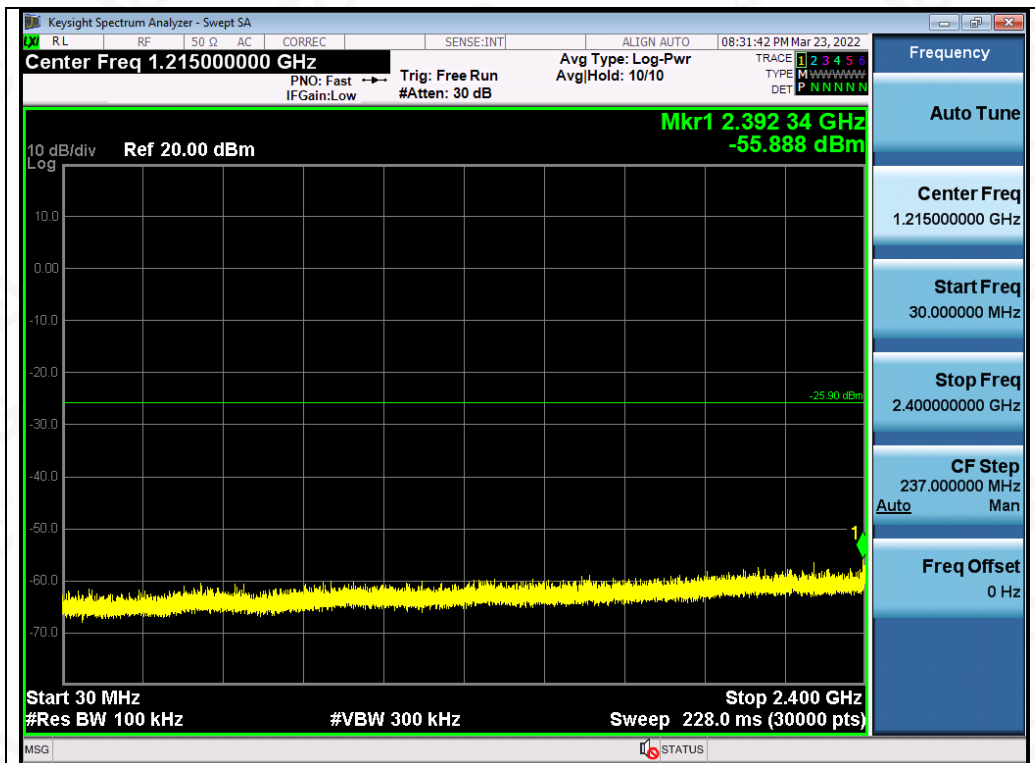
Test_Graph_802.11n20_ANT1_2437_MCS0_Lower Band Emissions
