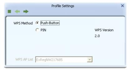
c. When the router's WPS status indicator led starts to flash and then click "Start PBC" button in two minutes.
