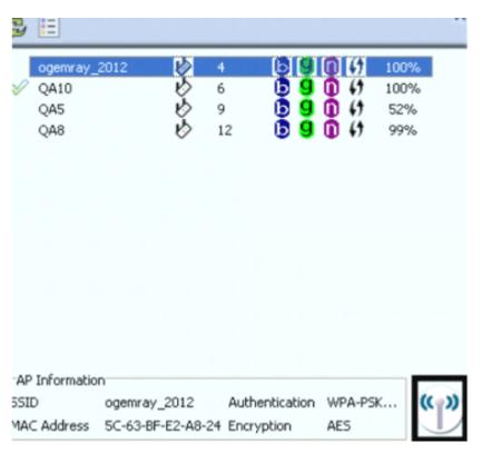
e. The Ralink Utility automatically detects and displays the security settings of the network to which you are connecting in the Profile Setting screens. If the Utility shows that WPA-PSK or WPA2-PSK security is detected as shown Below, click the right arrow to save your settings.
