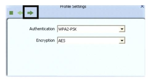
In the screen that displays, in the 'WPA Preshared Key' field ,type a security key, the same as that f. used by the AP or wireless router to which you are connecting. Click the right arrow to save your settings and connect to the network.
