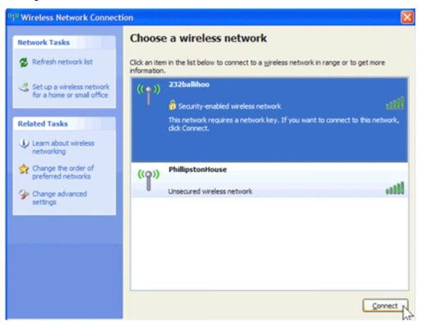
7) If the network security key hasn't been inputted before, Windows XP prompts you to enter the network's security key to access the wanted SSID. Type the encryption key that you wrote down earlier in both the Network key and Confirm network key boxes, and then click "Connect".
