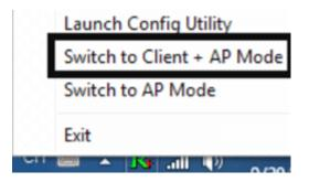
This mode lets you use the adapter both as a Soft-AP and client at the same time. Switch to this mode, you can let a wireless adapter be connect to a wireless (Soft-AP) with Internet connected, and let others adapter be indirectly connect to Internet via the Soft-AP wireless network.
