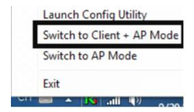
This mode lets you use the adapter both as a Soft-AP and client at the same time. Switch to this mode, you can let a wireless adapter be connect to a wireless (Soft-AP) with Internet connected, and let other adapter be indirectly connect to Internet via the Soft-AP wireless network.
