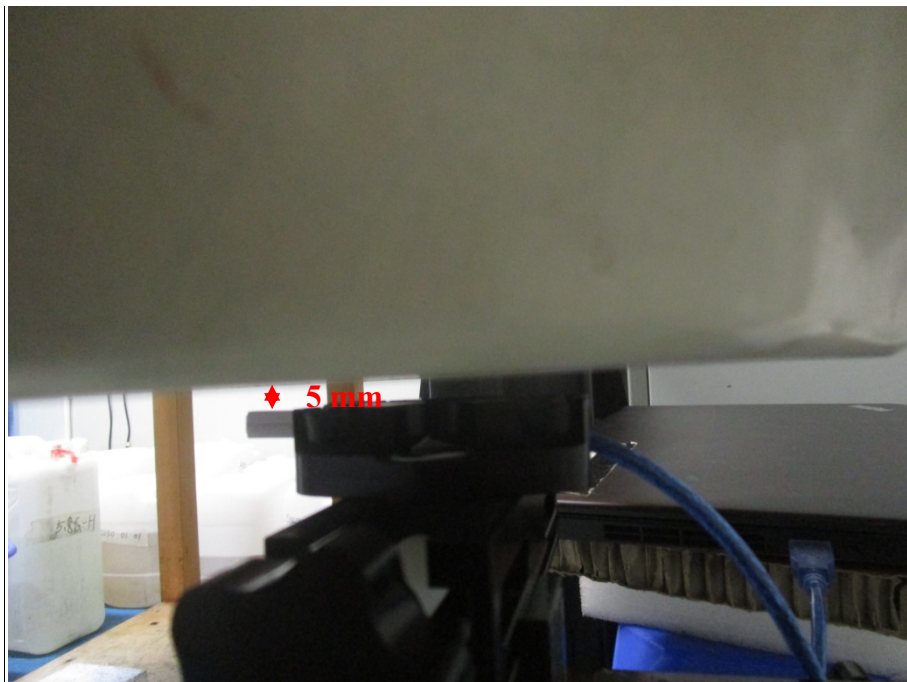
Horizontal-Down Setup Photo(5mm) _SAR Lab 1
