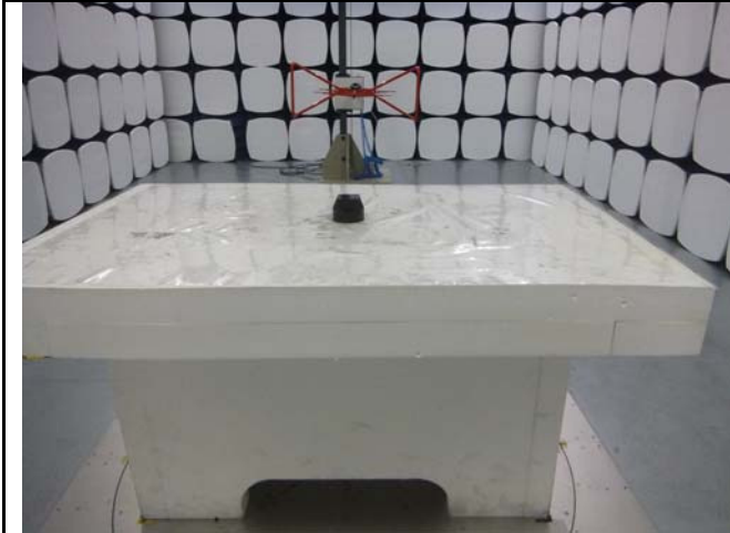
Radiated Spurious Emissions Test Setup Below 1GHz
