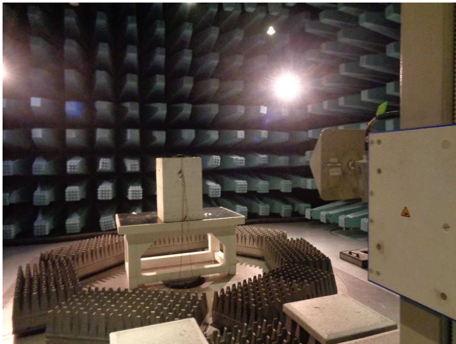
Figure 9.2-2: Radiated emission testing above 1 GHz
