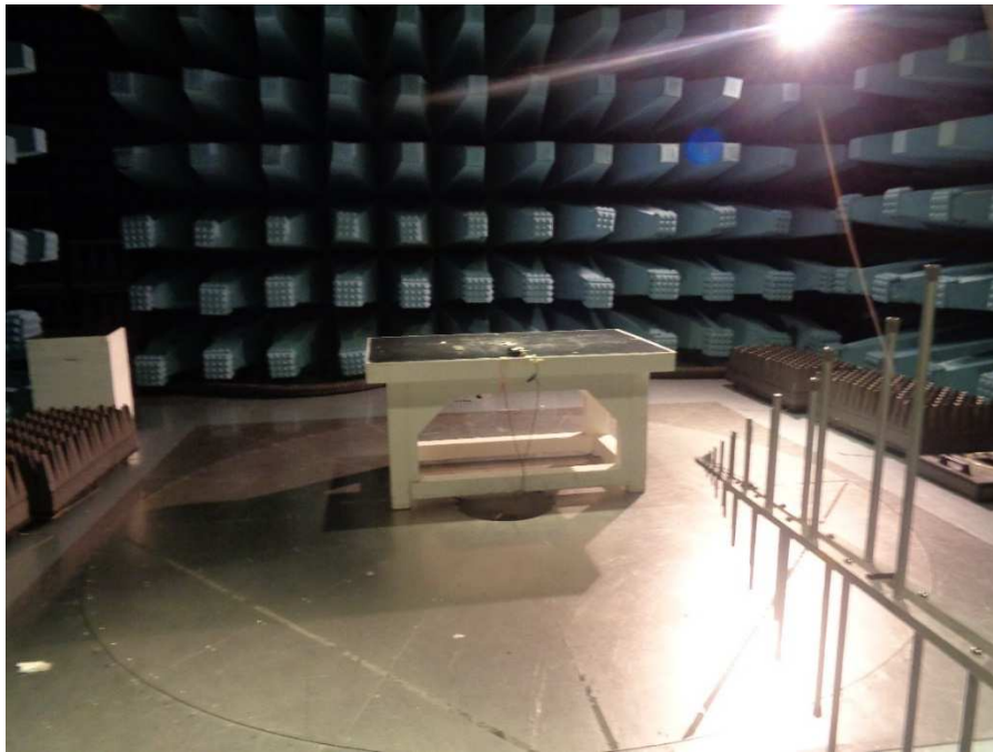
Figure 9.2-1: Radiated emission testing below 1 GHz
