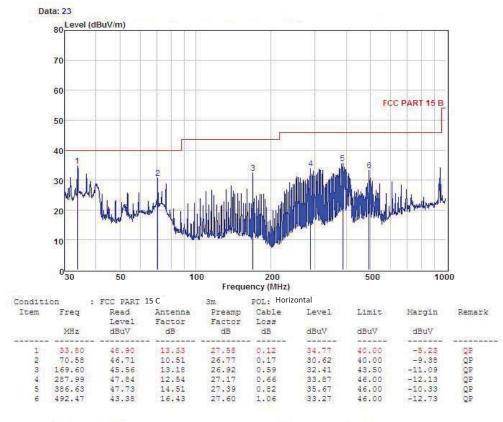
Remark: Level = Read Level + Antenna Factor - Freamp Factor + Cable Loss
