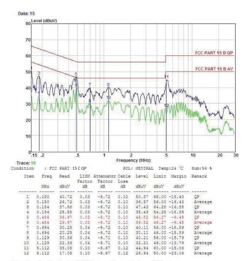
Remarks: Level = Read + LISN Factor -Attenuator Factor + Cable loss
