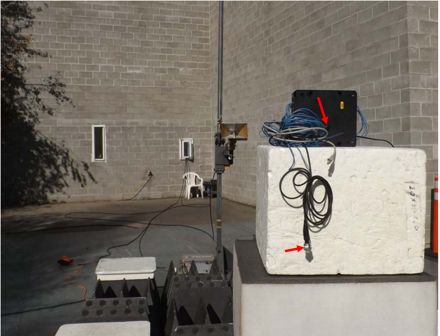
Figure E23.6 – Setup – Radiated Emissions, 1- 18 GHz
