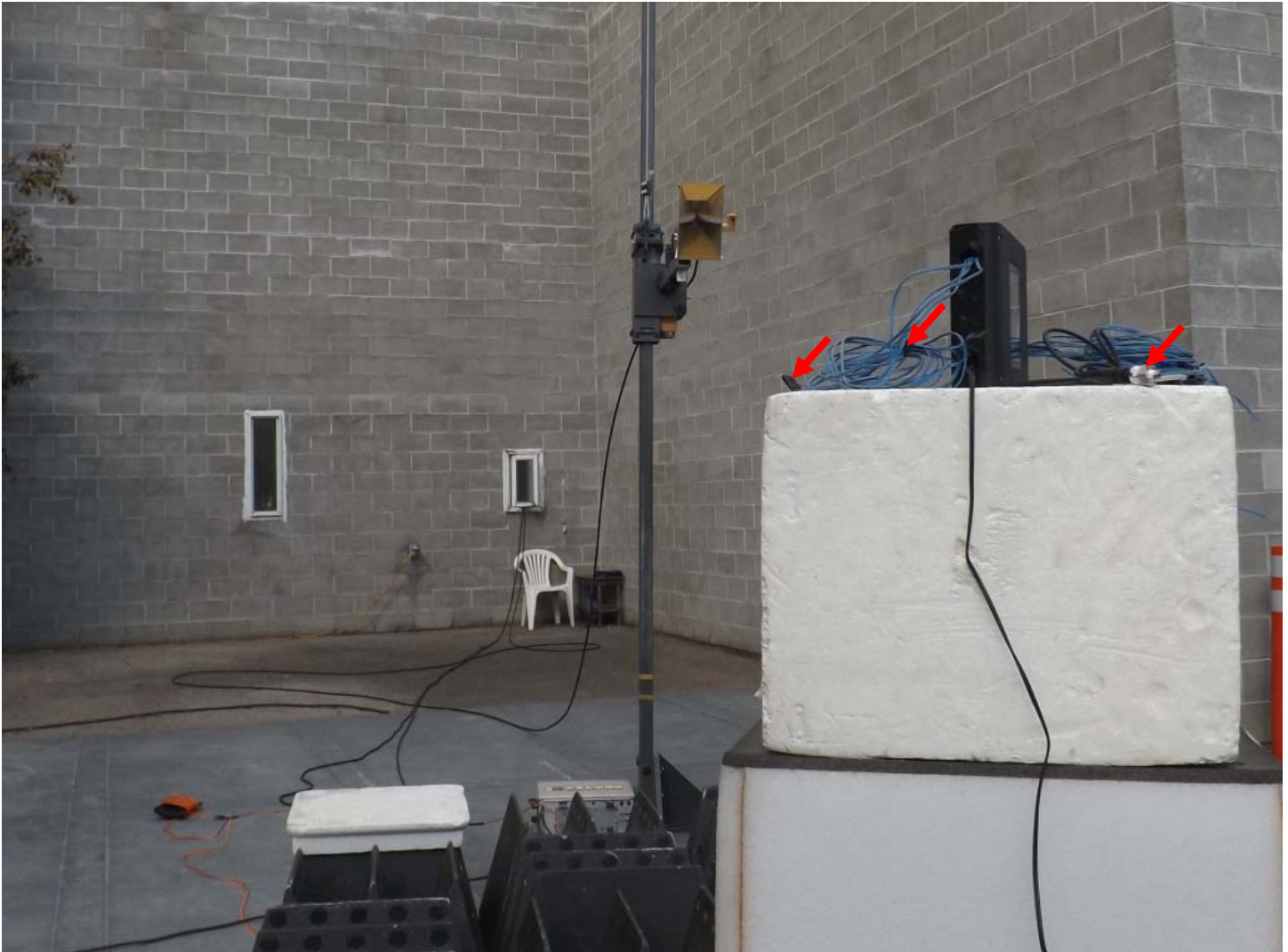
Figure E23.7 – Setup – Radiated Emissions, 1- 18 GHz
