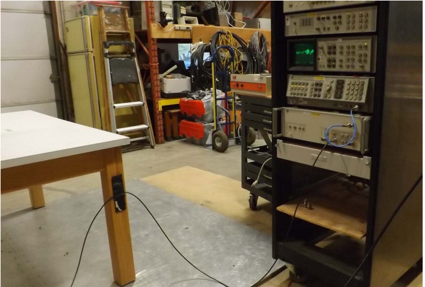
Figure E23.3 – Setup – Line Conducted Emissions
