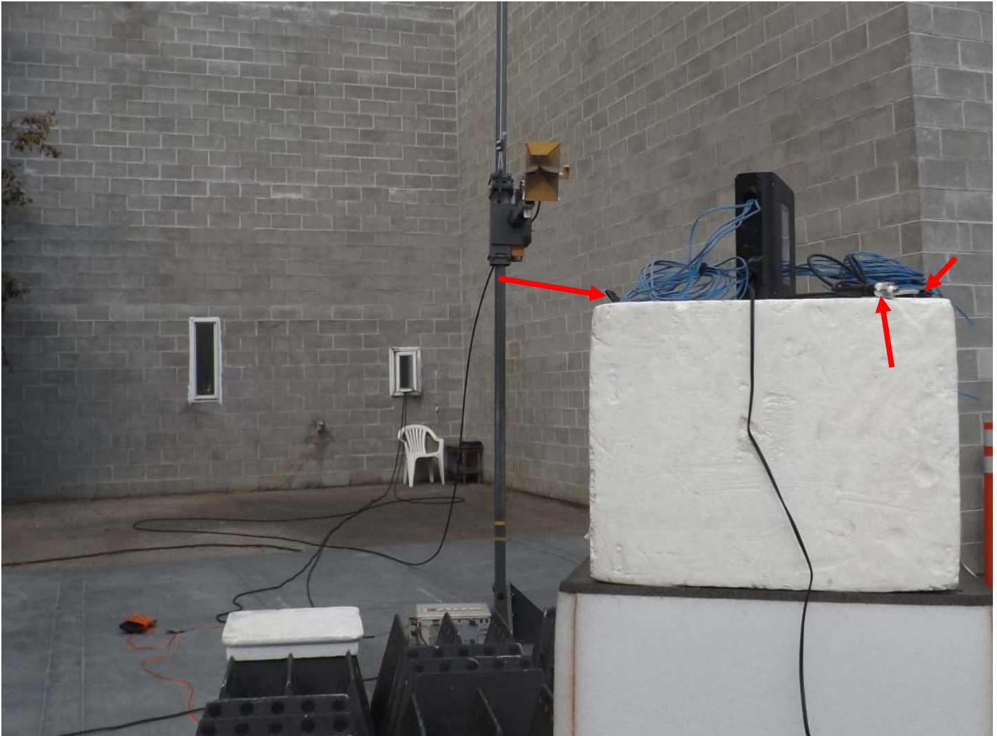
Figure E23.8 – Setup – Radiated Emissions, 1- 18 GHz
