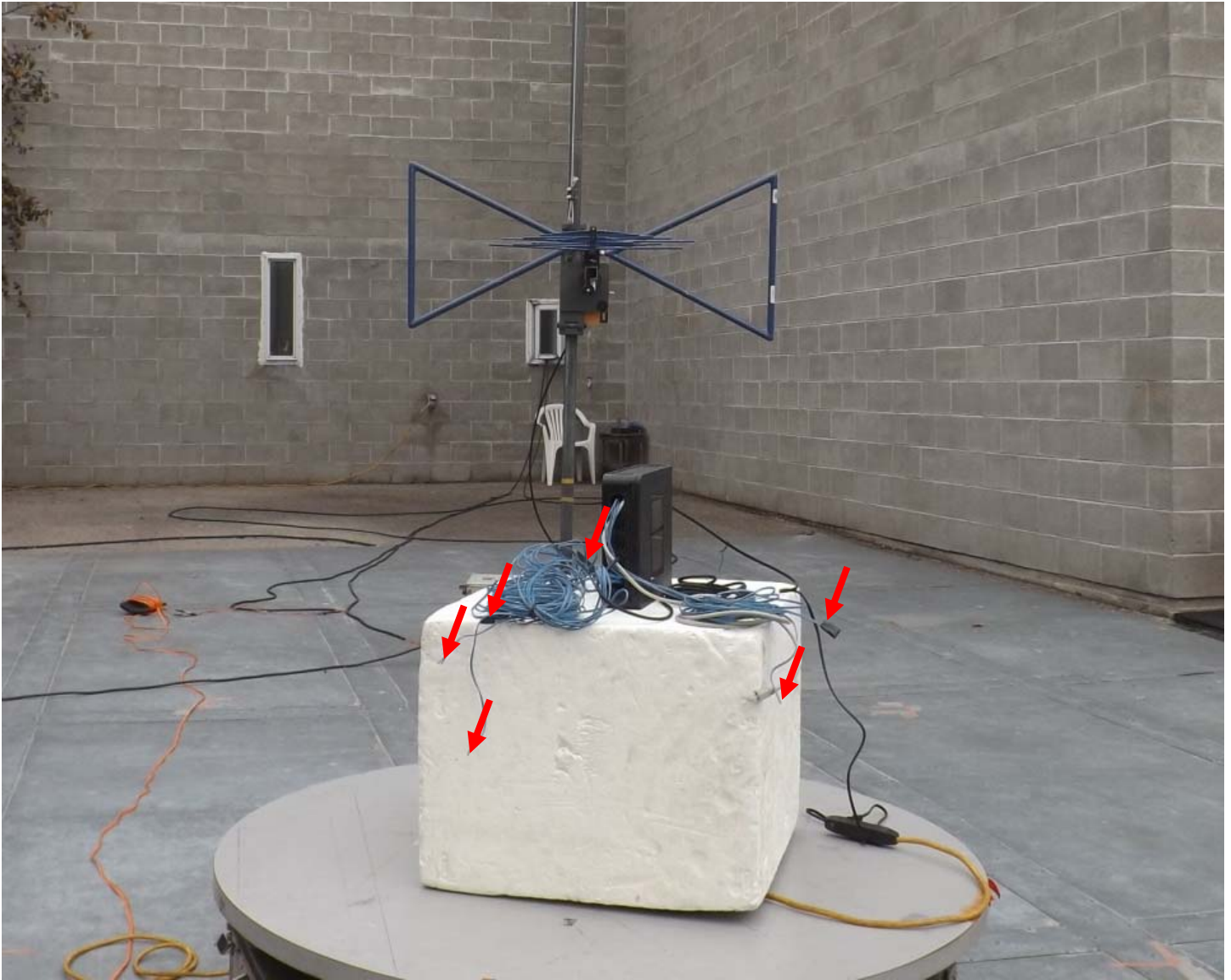
Figure E23.5 – Setup – Radiated Emissions, 30 – 1000MHz
