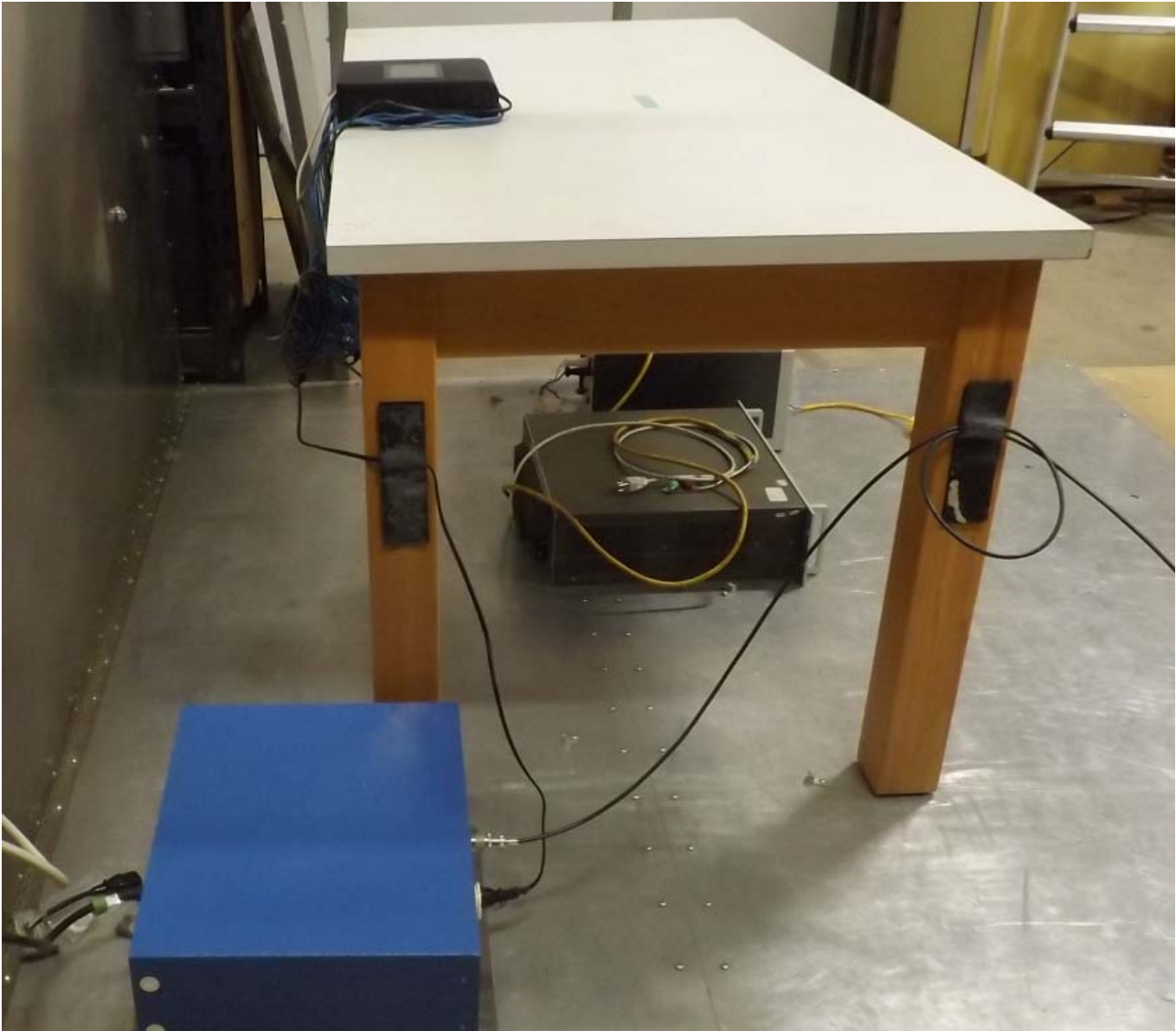
Figure E23.2A – Setup – Line Conducted Emissions
