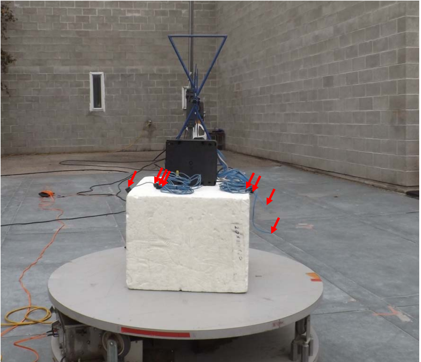
Figure E23.4 – Setup – Radiated Emissions, 30 – 1000MHz
