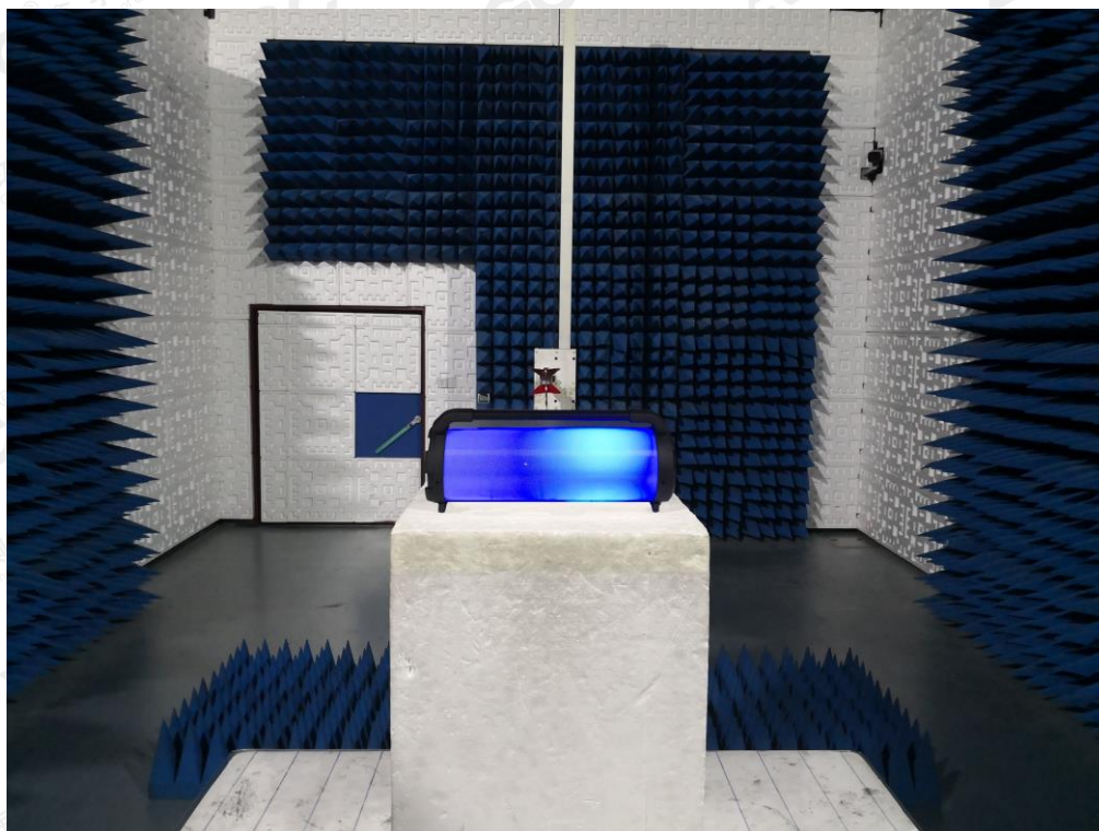
RADIATED EMISSION TEST SETUP ABOVE 1GHZ
