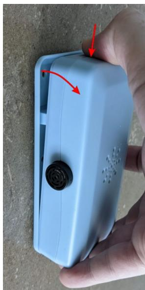
To “clip” a Sensor into a Backplate align the hook at the bottom of the Sensor with the pocket on the Backplate, then rotate in towards the Backplate until the Sensor locks into place (see right).
