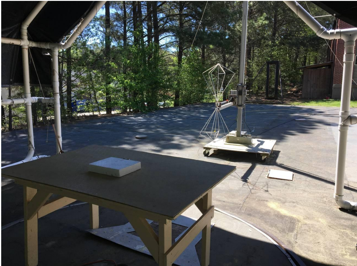
Figure 4. Radiated Emissions Test Configuration (30-200 MHz)
