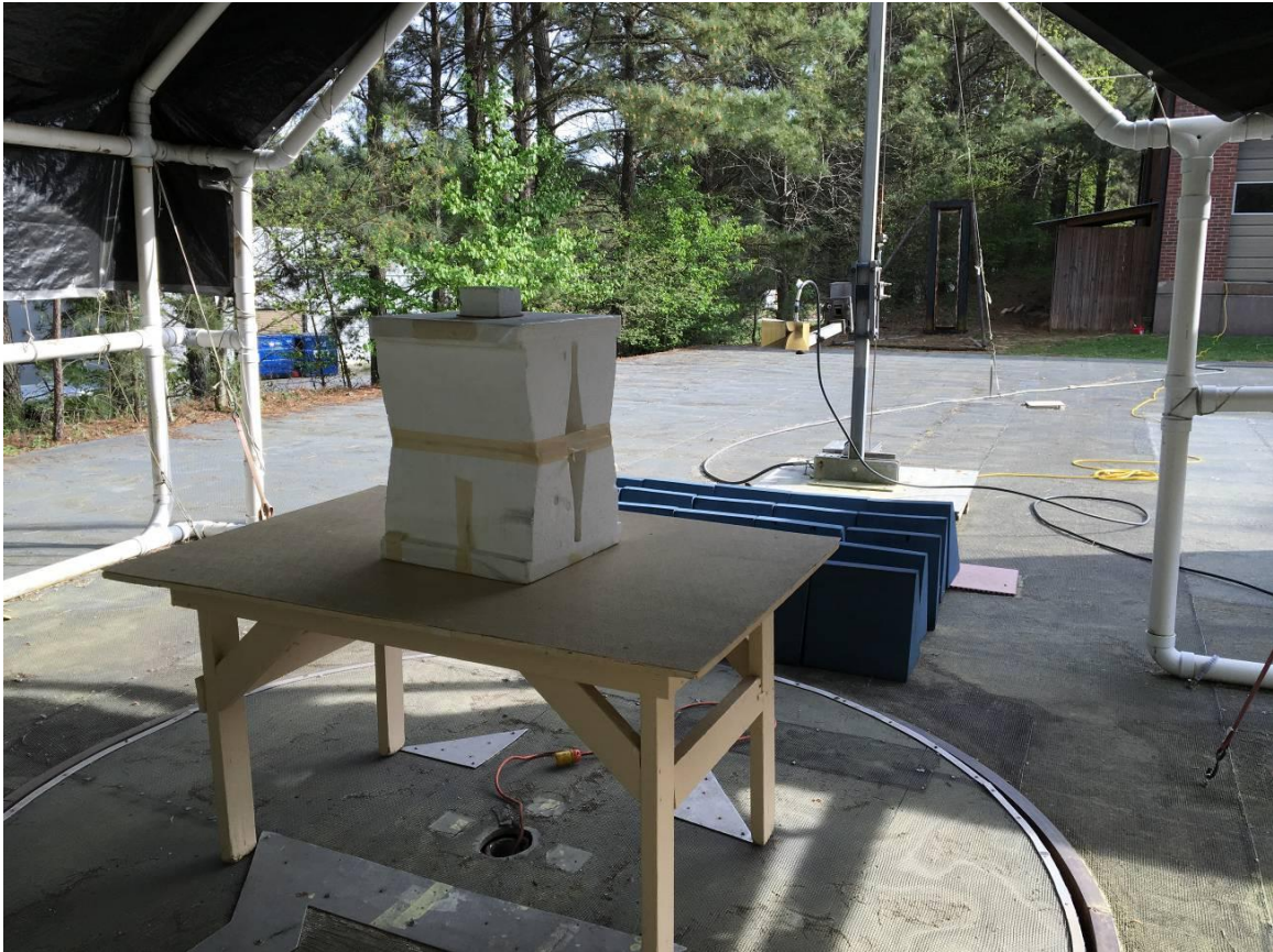
Figure 3. Radiated Emissions Test Configuration (above 1 GHz) Rear
