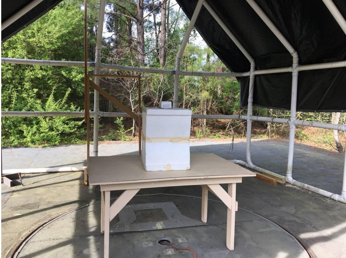
Figure 2. Radiated Emissions Test Configuration (above 1 GHz)
