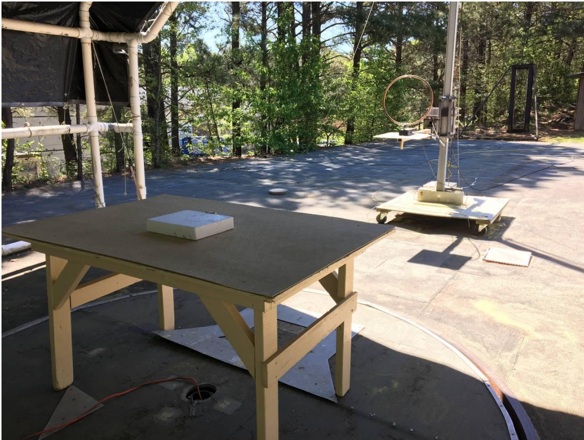
Figure 6. Radiated Emissions Test Configuration (0.150-30 MHz)
