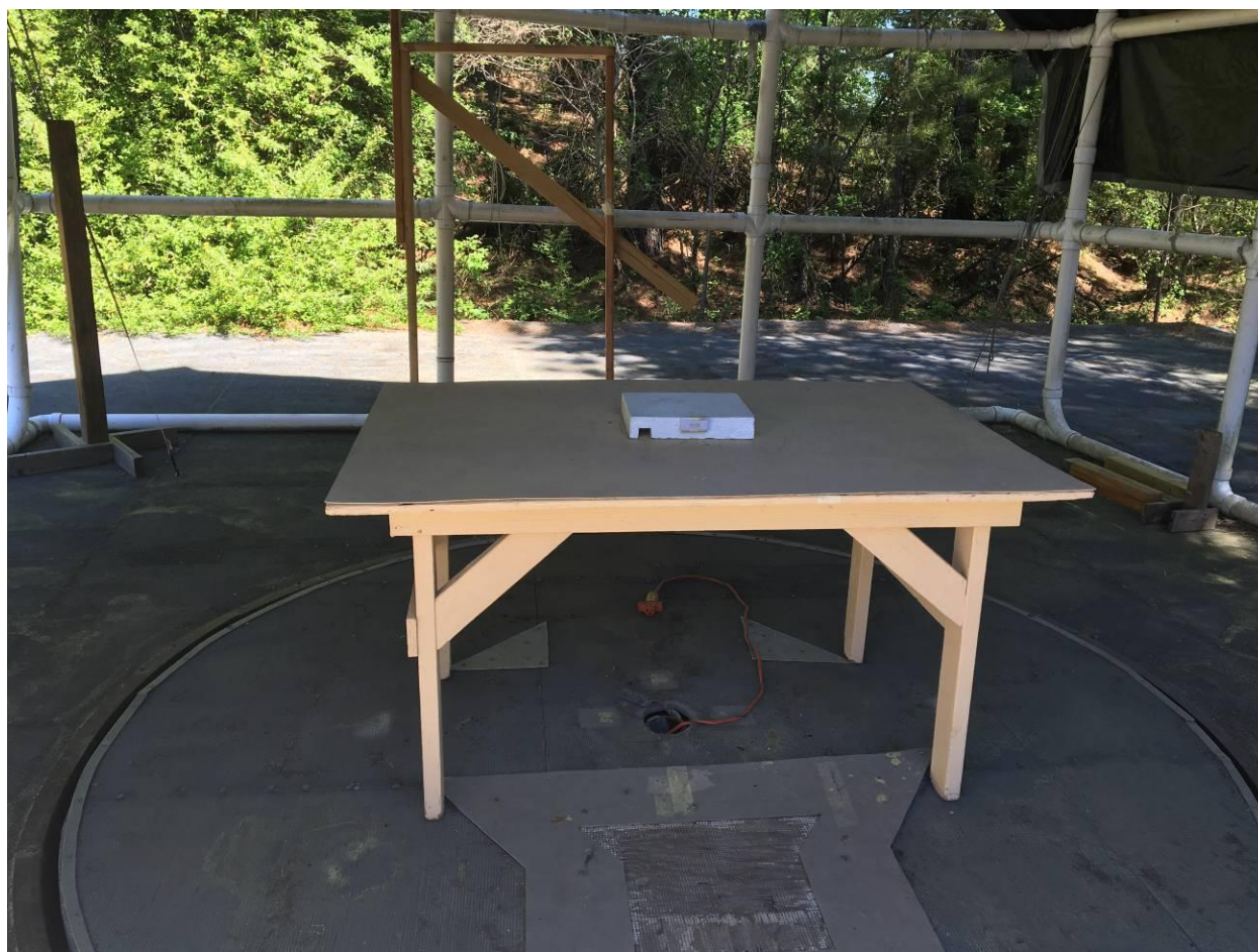
Figure 1. Radiated Emissions Test Configuration (below 1 GHz)
