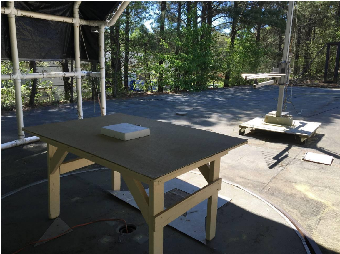
Figure 5. Radiated Emissions Test Configuration (200-1000 MHz)
