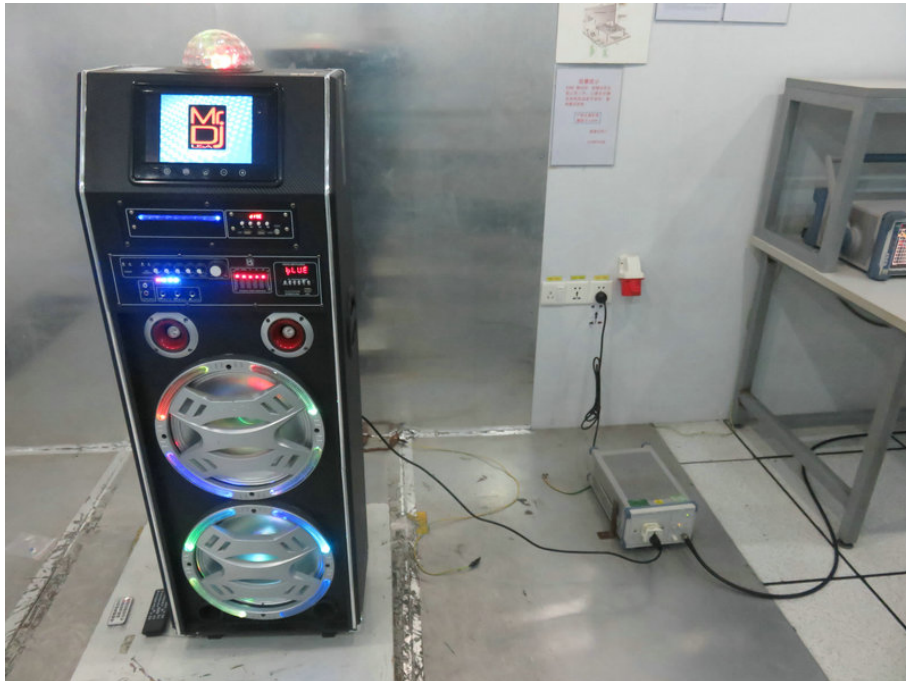
1 Photo of Power Line Conducted Emission Measurement
